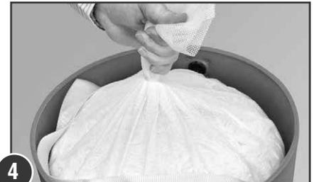
**4** Remove plastic bag and insert the filter bag (white netting with tied top) pushing it gently but firmly down to the base of the unit.
