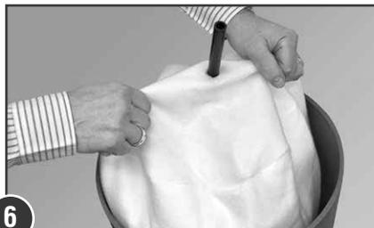
**6** Remove the plastic bag and insert the second filter bag (needle-felt bag with black inlet tube) and rest it on top of the retainers.
