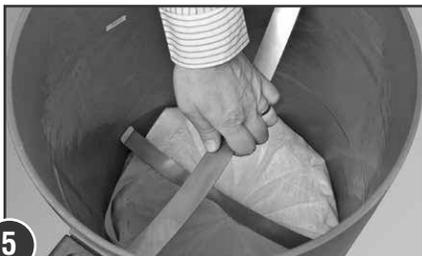
**5** Insert the metal retainer(s) with bent ends facing towards. Slide down until it touches the top of the filter bag. DO NOT compress the filter bag.
