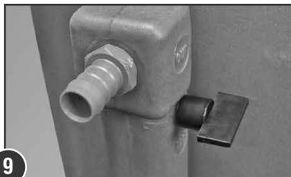
**9** Attach the twist off grab tap to the test point. Attach your outlet hose to the nipple above. Fill unit with water and check for leaks.
